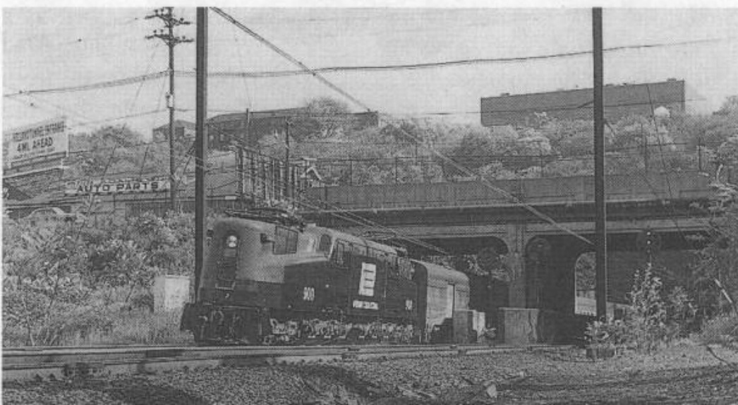
Train No. 2, "The Pennsylvania Limited," behind a stocky L-5 dc motor heads into Bergen Portal under the newly installed ac catenary. This extra-rare photo is dated September 25, 1932. (Smithsonian Institution) Below: Forty-one years later the name of the game is "Amtrak" and the name of the train is "The National Limited," powered by GG-1 No. 900 drawing 11,000 volts ac from that same catenary. Wires duck under U.S. Route I overpass. (Photo by author)
